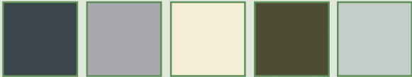
Anthracite Grey RAL 7016 White Aluminium RAL 9006 Cream RAL 9001 Quartz Grey RAL 7039 Light Grey RAL 7035
